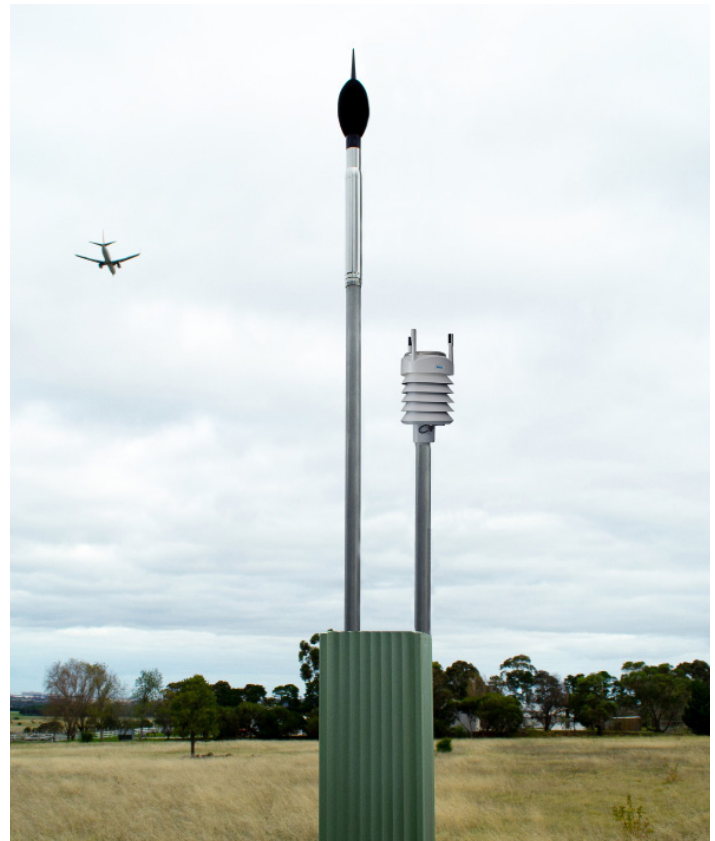
EMU set-up on site with Microphone and Weather Sensor
